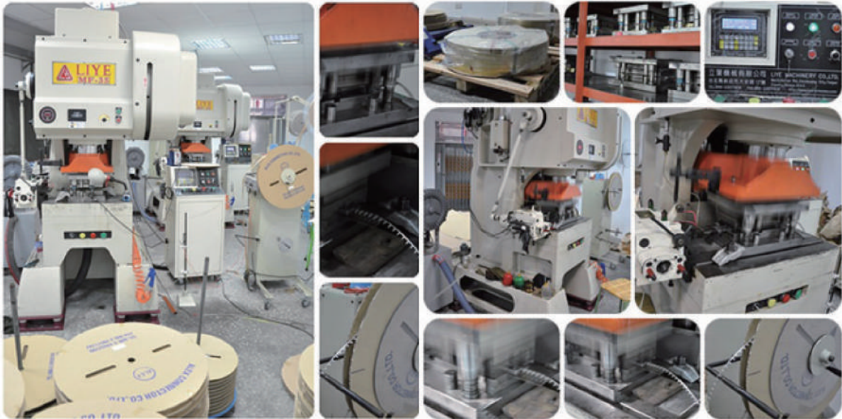
Stamping process and die for connector terminal.
