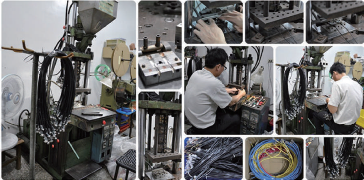
Modeling process and die for connector terminal.
