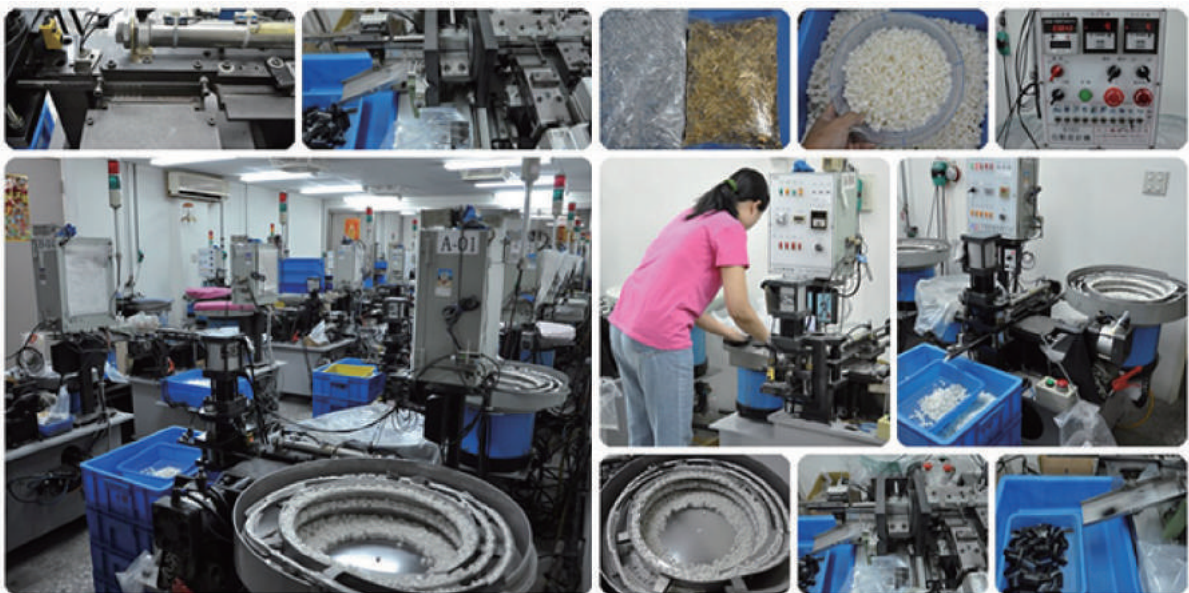
Pin Inserting process and die for connector terminal.
