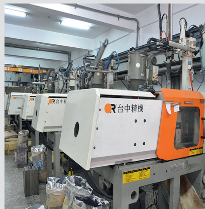
Plastic Injection Plant
